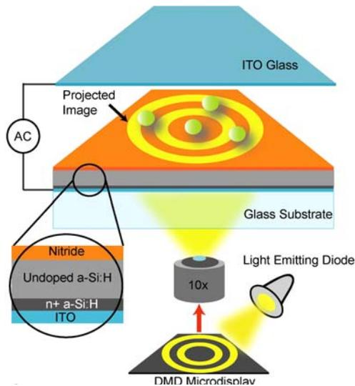
Figure 1 Schematic of optoelectronic tweezers (OET)
